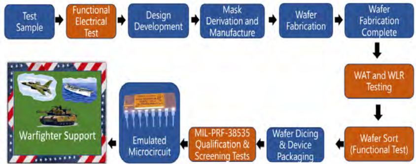
Figure 1. Electrical & QA Testing Overview.
